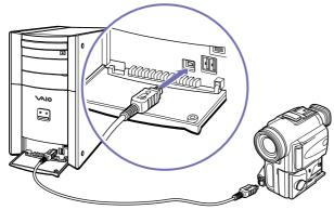
On Sony digital video cameras, connectors labelled **DV Out**, **DV In/Out** or **i.LINK**<sup>TM</sup> are i.LINK<sup>TM</sup>-compatible.
